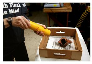
Hold the outer tube (printed one) with one hand; twist the inner tube (see photo above) while pumping to spray the object you wish to coat. Keep the Mini Flocker 8" to 10" from surface and as close to 90 degree to the object as possible.
