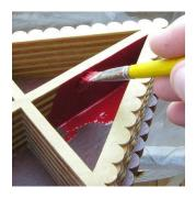
Flock It! Suede-Tex undercoat adhesive can be brushed, sprayed or rolled onto the area to be coated.
