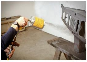
Set your compressor at 10 to 15 psi (it is okay to go up to 20 psi, but the flocking fibers will spray out of the canister more quickly requiring frequent refills). Hold the gun on a slightly downward angle (see photo) and depress the trigger at the handle. Keep the AASG 8" to 10" from surface and as close to 90 degrees to the object as possible.
